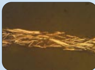
Metal flakes in paints leave substantial pockets of non-conductive polymer, compromising conductivity of the enclosure.
