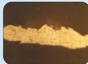
The ECOPLATE process applies a tenacious, pure metal film with <6% porosity, ensuring very high conductivity and reliability.
