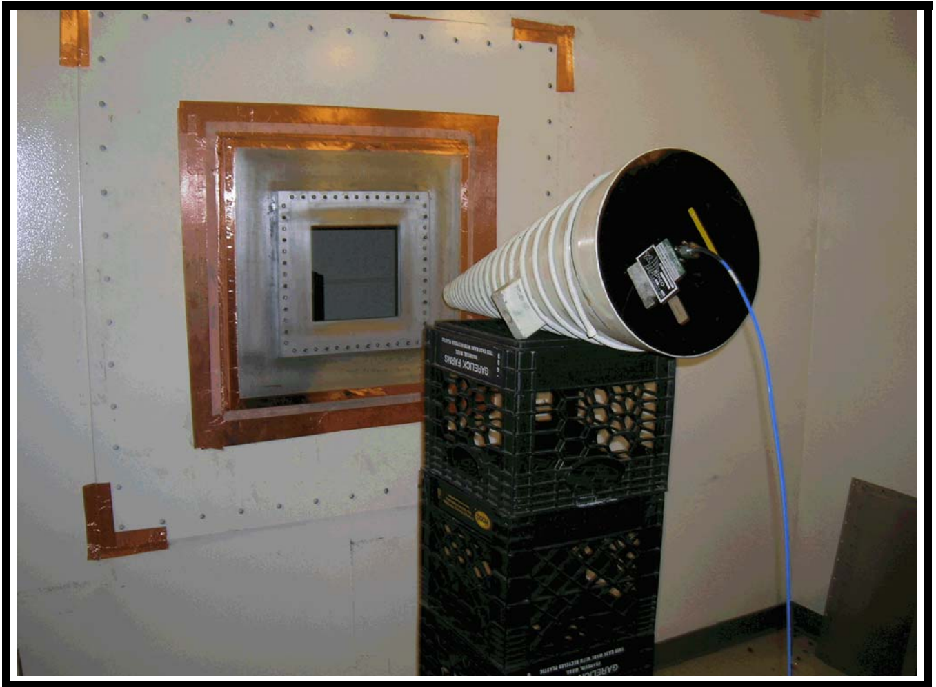
Photograph Description: Basic Thru-Hole Open Reference Setup 200MHz to 1GHz
