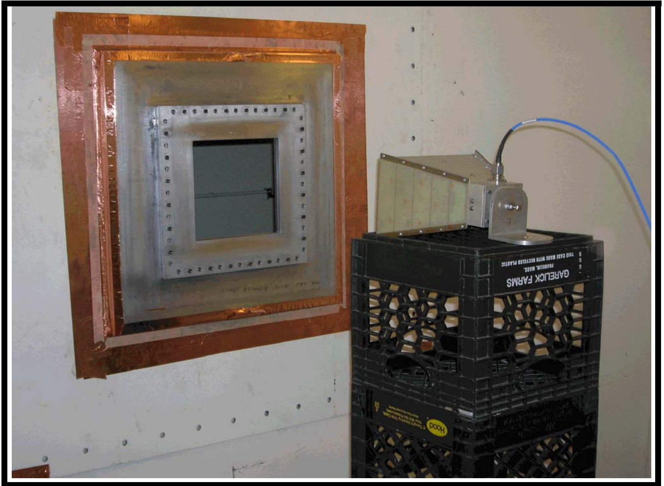
Photograph Description: Basic Thru-Hole Open Reference Setup 1GHz to 18GHz
