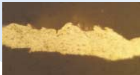
The ECOPLATE process applies a tenacious, pure metal film with <6% porosity, ensuring very high conductivity and reliability.
