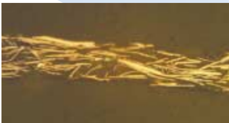
Metal flakes in paints leave substantial pockets of non-conductive polymer, compromising conductivity of the enclosure.
